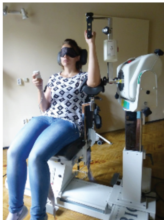
Figure 1. Elbow joint position sense measurement (passive mode) – examinee holds the Biodex moving arm which allows the elbow to be in continuous passive motion, the transducer is placed parallel to the forearm, on the Biodex moving arm; the examinee holds the remote in the contralateral hand.
